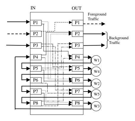
**Figure B.10** Implementation of 7-to-2 partial cross configuration with 2 generators for background traffic in latency measurements.
