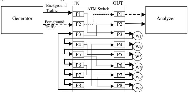
**Figure 3.5**: A scaleable test configuration for measurements of MIMO latency using only two generator analyzer pairs with 8-port switch and 7-to7 straight configuration for background traffic
