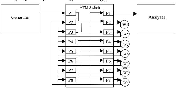
**Figure 3.3**: A scaleable test configuration for throughput measurements using only one generator/analyzer pair with 8-port switch and 8-to8 straight connection configuration.
