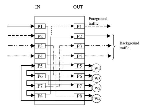
**Figure B.8** Implementation of the 7-to-7 straight configuration with 3 generators for background traffic in latency measurement.
