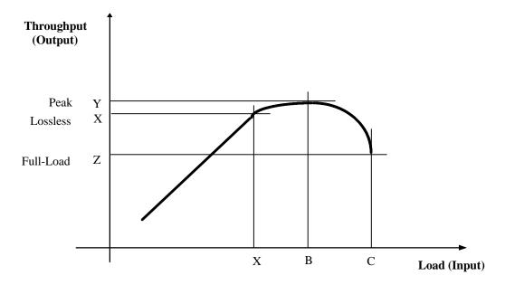
Figure 3.1: Peak, loss-less and full-load throughput
