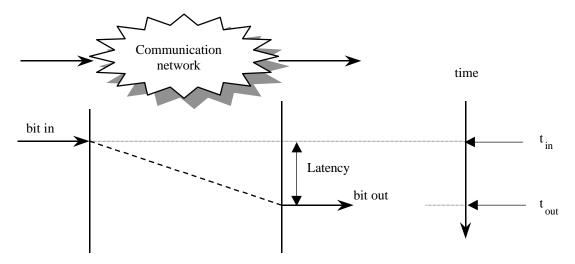
Figure A.1: Latency for a single bit
