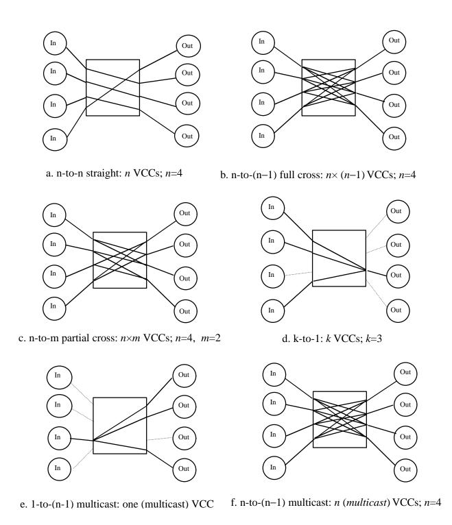
Figure 3.2: Connection configurations for foreground traffic
