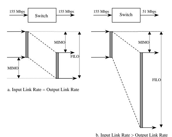
**Figure A.12**: FILO Latency as User Perceived Delay
