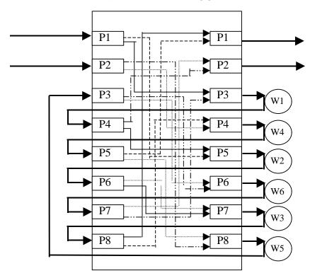
**Figure B.9** Implementation of 8-to-2 partial cross configuration with 2 generators for foreground traffic
