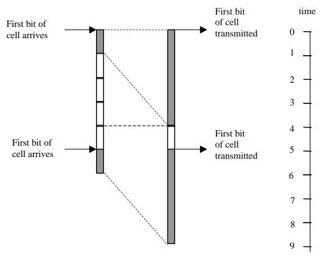
**Figure A.7**: Zero Delay Switch Operations, no Cell Waiting Case (Input rate > Output Rate)
