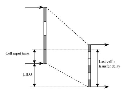
**Figure A.11**: LILO Latency Calculation (Input rate ≤ Output Rate)
