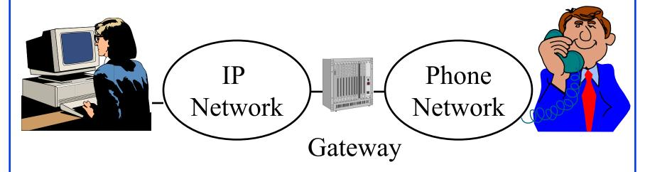
■ Need a gateway that connects IP network to phone network (Router to PBX)
