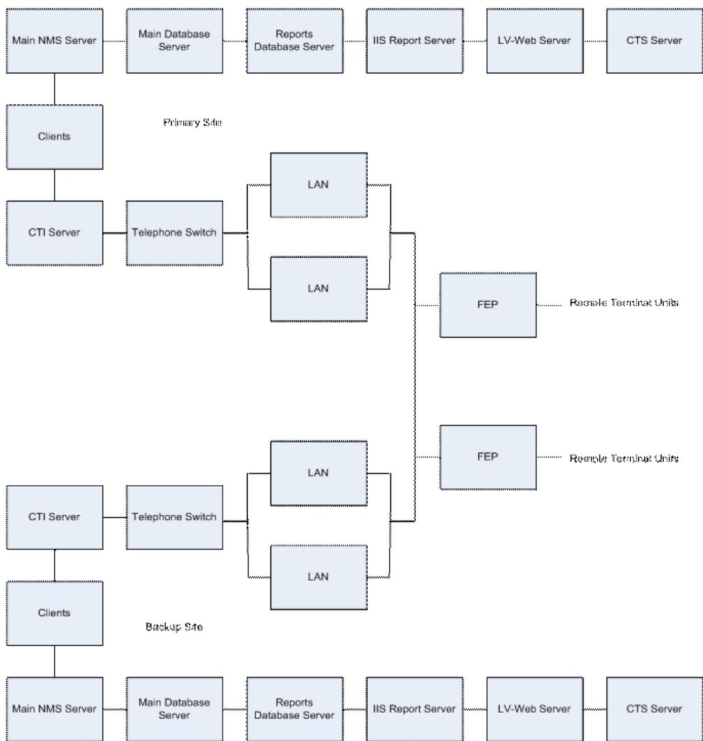
Figure 4: Model of a SCADA/OMS/DMS Control System
