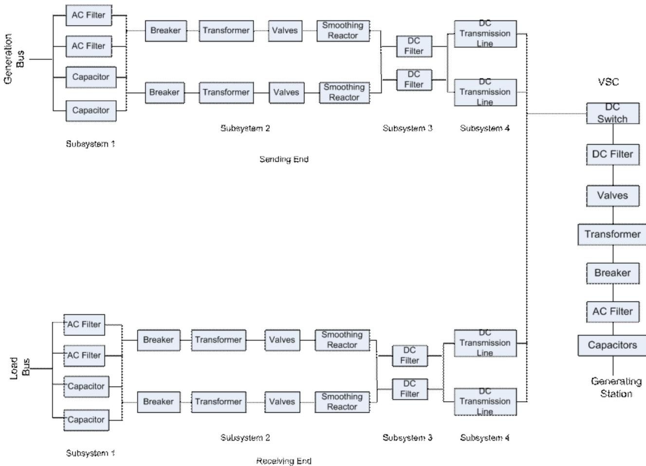
Figure 3: Model of a HVDC Transmission System
