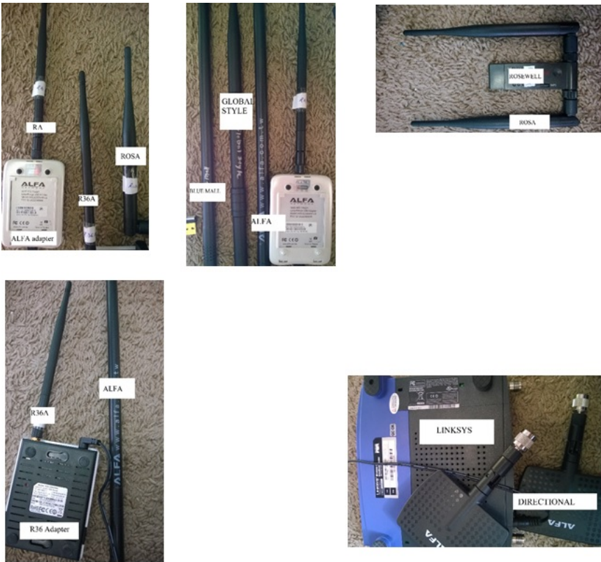
FIGURE 1 (left to right, top to bottom) ALFA Adapter with RA, R36A and ROSA Antennas; ALFA Adapter with Blue Mall, Global Style and ALFA antennas; ROSEWILL adapter with ROSA antenna; R36 adapter with ALFA antenna; Linksys router with directional antennas
