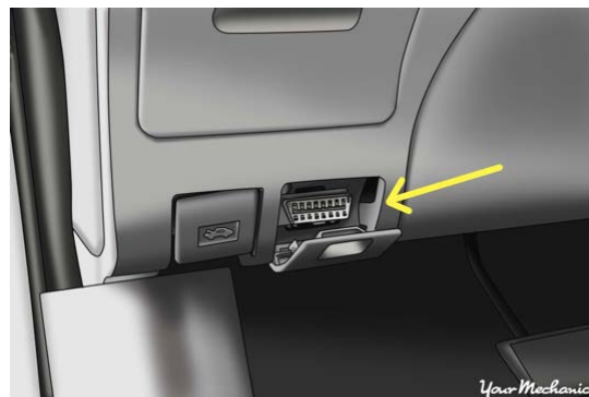
Figure 4: OBD-II Automotive Diagnostic Port.
