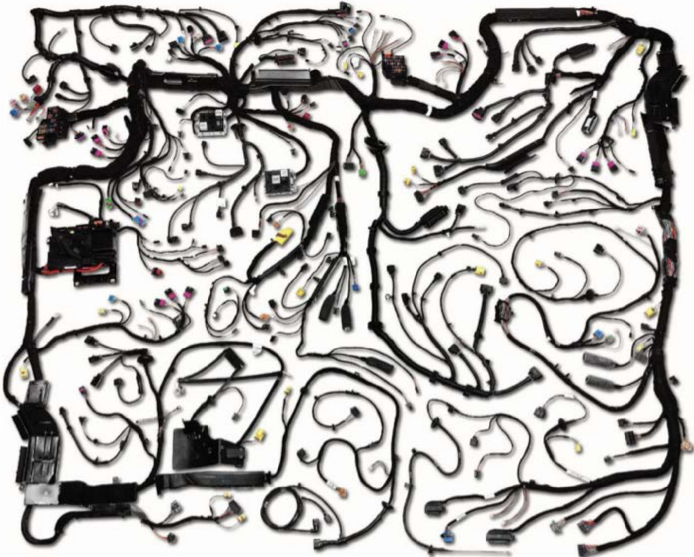
Figure 1: A typical wiring harness for a car.
