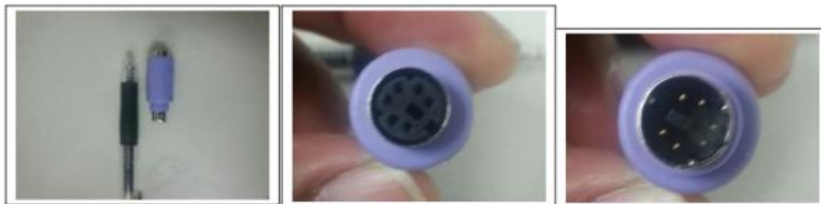
Figure 14: Skimming devices found on six registers at a Nordstrom department store in Florida[4. Brian Krebs]
