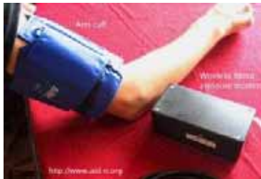
Figure 8: UVA/AID-N wireless blood pressure cuff [CodeBlue]
