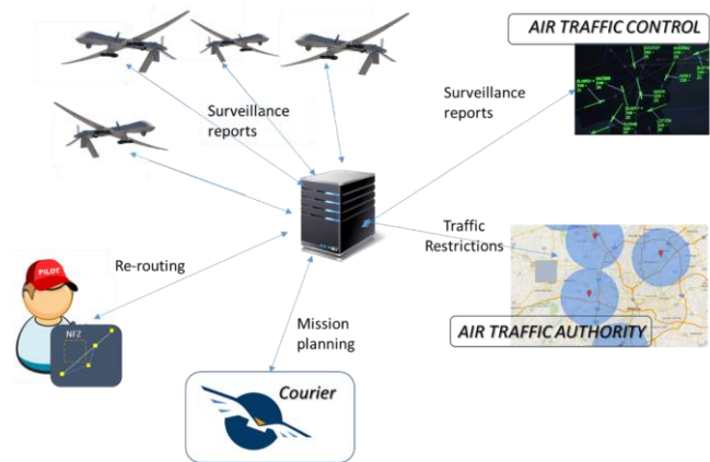
Figure 9 - ADS-IP Surveillance System
