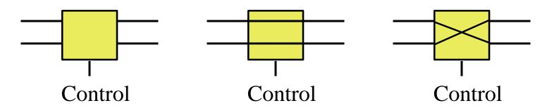
$\square$  Larger switches can be built out of  $2 \times 2$  switches
