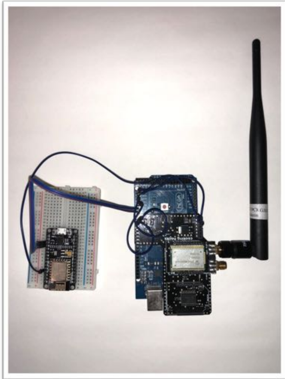
Figure 6.5: Arduino MEGA, Connection Bridge, Cooking Hacks LoRaWAN Module, and ESP-12e Setup
