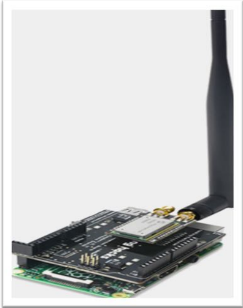
Figure 6.1: RPI3, Connection Bridge, & Cooking Hacks LoRaWAN Module Setup
